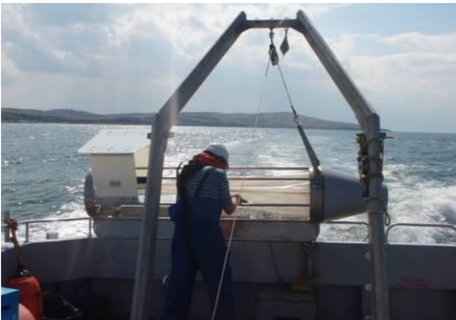
Figure 2.2 : Deploying the Gulf™ plankton sampler over the stern of the SeeKat C.
